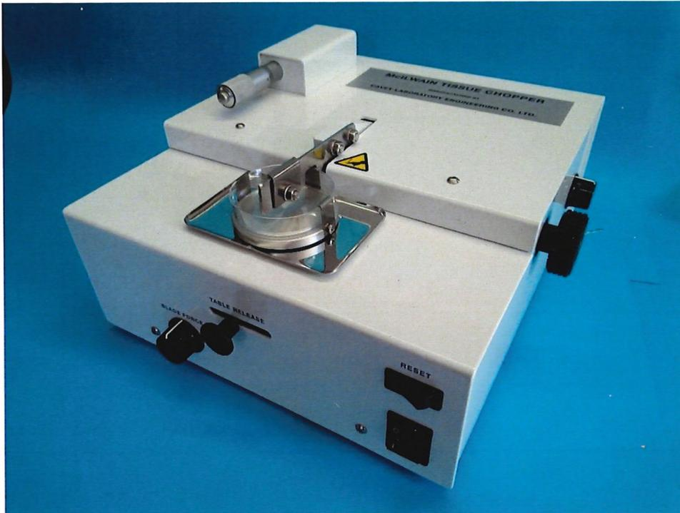
This apparatus has been designed to prepare pieces of tissue for metabolic experiments and to be especially applicable to small and irregular specimens available at biopsy or from small organs. Its special features are to cause much less disturbance of cell structure than homogenisers or blenders and to be applicable to fragments that would be difficult or impossible to cut by ordinary methods. Typical applications are to liver, kidney and various parts of the central nervous system.
